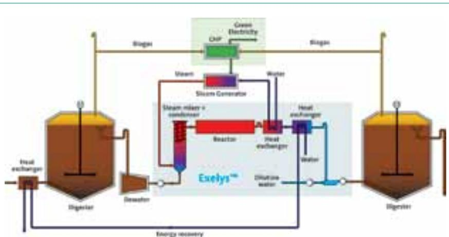
Figure 5: The DLD™ (digestion-lysis-digestion) process configuration uses the Exelys™ process to increase biogas production, maximize electricity production, and minimize the volume of sludge requiring disposal.
