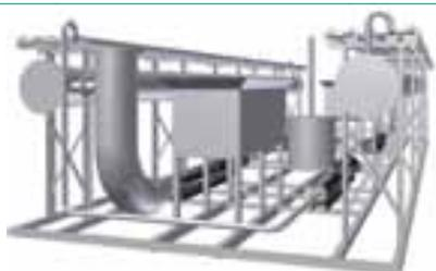
Figure 4: The Exelys™ thermal hydrolysis process increases bio-mass concentration, thereby reducing the volume to be heated for anaerobic digestion.
