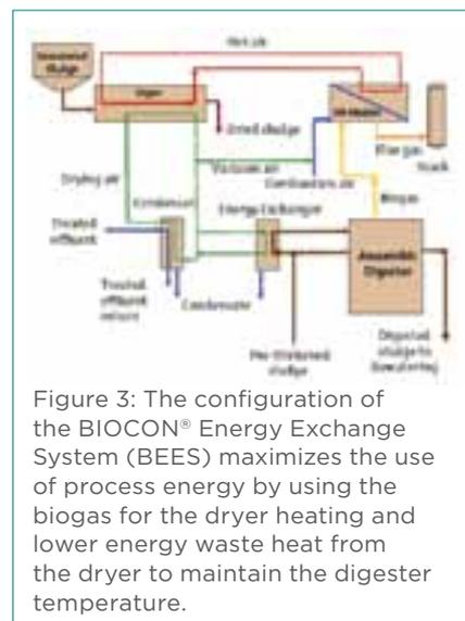
Figure 3: The configuration of the BIOCON® Energy Exchange System (BEES) maximizes the use of process energy by using the biogas for the dryer heating and lower energy waste heat from the dryer to maintain the digester temperature.
